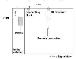
The IR IN input allows you to control the DTR-8.3 from the remote zone (Zone 2) with the remote controller even though the remote zone may be on the other side of the building from the main zone. The diagram below shows how to make the proper connections for the remote zone.
